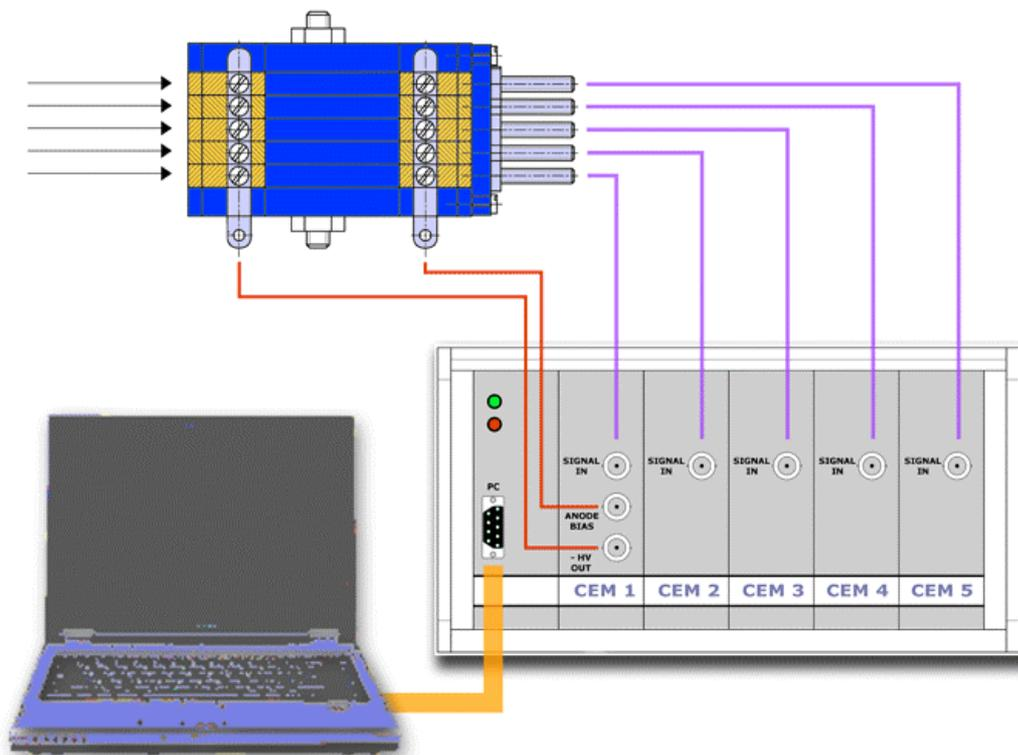
Fig. 2: CEM-array with negative high voltage
