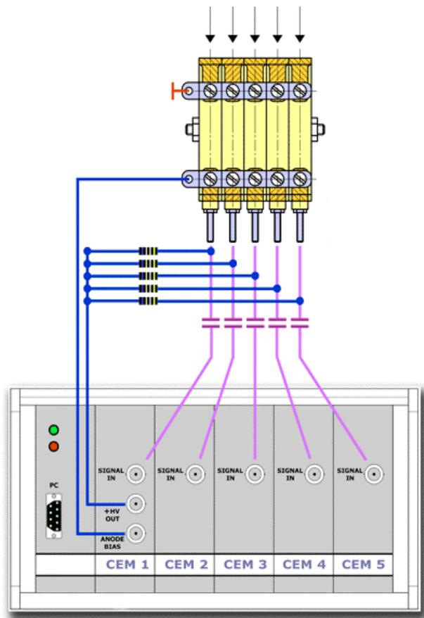
Fig. 3: CEM-array with positive high voltage
